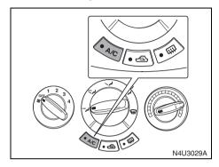
If your vehicle has air conditioning, follow these steps to use the system. Start the engine and set the fan control knob to the desired speed. The air conditioning compressor does not operate when the fan control knob is in the off position. Press the air conditioning button to turn the air conditioning system on. When this button is pressed, the indicator light on the button will come on to let you know the air conditioning is activated.
